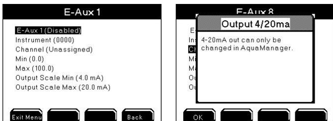
4/20mA menu configuration information is provided at AquaManager Help. See AquaManager Help contents>working with nodes>expansion modules>ioem expansion module>configure ioem 4mA-20mA output to a 5X00 system bookmark. Configure 4/20mA outputs at sensor system tabs in AquaManager. 4/20mA configuration fields are located at the bottom of all sensor system tabs.
