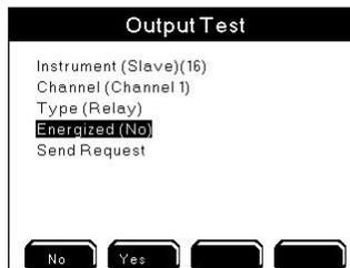
8. Scroll and select Send Request. at 5X00 Run Screen to send a command to the local, or networked, instrument to trigger configured output test condition.
