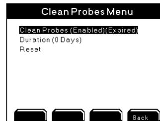
Reset Clean Probe timer at the **Msg's** menu or the Reset Clean Probes menu.
