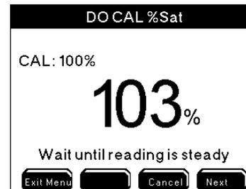
9. After 10 minutes, verify that the DO reading shows no significant change for approximately 30 seconds. Then, press **Next** to complete the calibration OR press **Cancel** to abort the calibration without saving.
