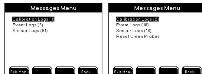
A Reset Clean Probe message will appear at the Msg's Menu if the clean probe timer expires. Selecting "Yes" at "Are you sure?" resets the clean probe timer to the user configured number of days.
