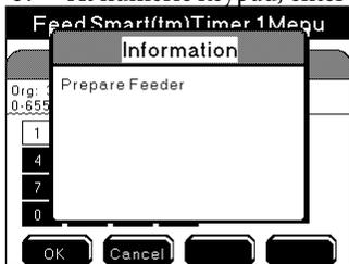
6. Press **OK** for feed timer relay to energize for configured run test time. Countdown of relay “on” time is displayed.
