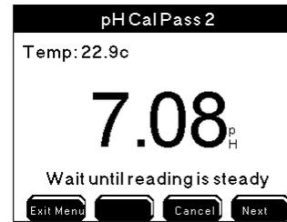
9. After one minute, verify that the pH and temperature values show no significant change for approximately 30 seconds. Then, press **Next** to continue the calibration OR press **Cancel** to escape calibration and return to calibration menu without saving.
