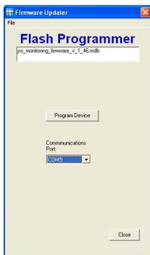
6. AquaManager Program Folder includes the latest version of instrument firmware. The latest firmware is stored as an .mdb file in the PC Program Files>AquaManager>Firmware. At AquaManager, Firmware Updater>File>Load Firmware Database. Locate and load this file into the Firmware Updater.
