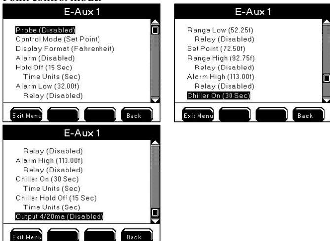
Control relays configured in the Set Point control mode energize when a user configured control value is received from the input device and is processed by the 5200A.
