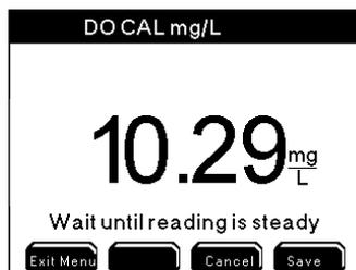
8. After one minute, verify that the DO value shows no significant change for approximately 30 seconds. Then, press **Next** to complete the calibration OR press **Cancel** to cancel the calibration without saving.
