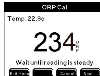
9. After one minute, verify the ORP and temperature values show no significant change for approximately 30 seconds. Then, press **Next** to complete calibration OR press **Cancel** to abort the calibration and return to calibration menu without saving any changes.
