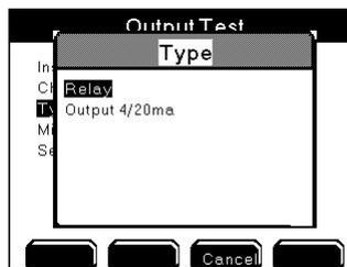
6. 4/20mA outputs test an IOEM 4/20mA output channel. For 4/20mA output test, configure a Milliamp value. The Milliamp range is 0.00 to 21.00.
