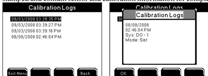
Certain calibration data is not available at the 5200A. Use AquaManager to view and save calibration data to the PC. In addition to sensor system, time, date, and calibration method, AquaManager calibration logs include user input 1, user input 2, and the original and new slope/offset information when applicable.
