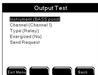
3. at Instrument menu. Device Address menu opens. Scroll and select networked instrument whose relay or channel is to be tested.
